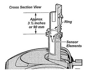
2. As indicated by the illustration, the two dirt sensor elements are located on the inside of the swivel, approximately 3½ inches/90 mm down, (note the arrows). Each element should be cleaned periodically. To reach the sensor elements, use a small brush such as a bottle brush. Brush each sensor element several times to remove dust and dirt.
