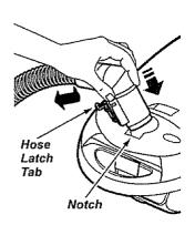
1. Line up the hose latch tab and notch in canister hood and insert hose into canister until it snaps in place.
