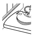
Active brush edge cleaners are on both sides of the POWER-MATE™. Guide either side of the POWER-MATE™ along base-boards or next to furniture to help remove dirt trapped at carpet edges.
