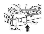
6. Lift agitator assembly out and remove worn belt.
