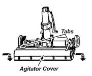
5. Line up front of cover and base. Rest cover on front edge of base as shown.
