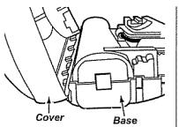
7. Tilt cover to back. Press cover firmly until side and rear tabs snap into place. Turn POWER-MATE™ upside down and replace two (2) cover screws.
