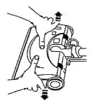
4. To remove cover, grasp the sides and pull out.
