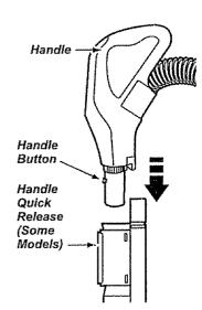
2. Insert handle into wand until lock button snaps in place. Be sure hose is not twisted.
