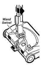
The swivel, located on the POWER-MATE™, allows you to turn the handle to the left side to reach farther under low furniture.
