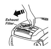
down until it snaps into place. Place the new filter into the motor cover with the **grey** edge down.
