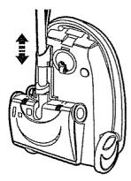
The flange allows the wands and POWER-MATE™ to be stored with the canister to conserve storage space. The canister must be stored on end for this feature to be used.
