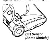
The lights give you an indication of the amount of dirt particles that are passing thru the sensor on its way to the dust bag.
