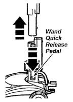
2. Press wand quick release pedal with foot and pull the wands straight up out of POWER-MATE™.
