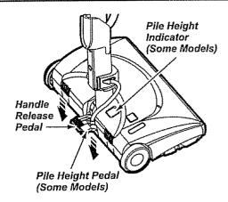
**3.** Lower wand from upright position by pressing on the handle release pedal.
