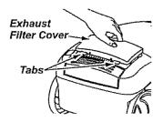
4. Replace the exhaust filter cover by engaging the two tabs on the rear and pushing down in front until it snaps closed.
