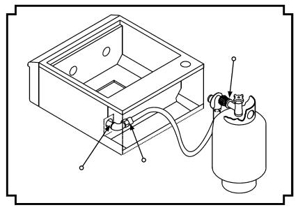
Figure 11-2 - Leak testing points when using L.P. gas.
