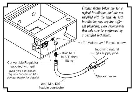
Figure 8-1 - Typical attachment for using natural gas.
