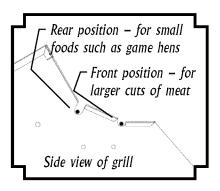
Figure 16-2 - Dual position rotisserie system.
