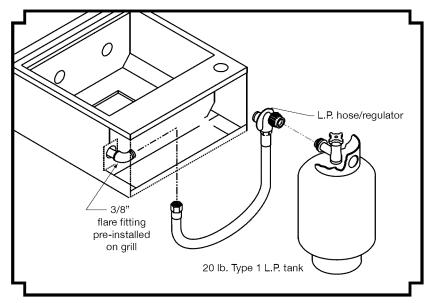
Figure 9-1 - Typical attachment to L.P. tank.
