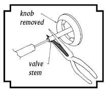
**Figure 14-1** - Adjusting brass burner low heat setting.
