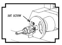
Figure 19-2 - Air shutter set screw location on burner
