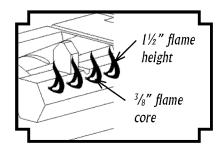
**Figure 19-1** - Showing proper flame characteristics.
