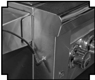
Figure 16-1 - Rotis motor power jack located on grill
