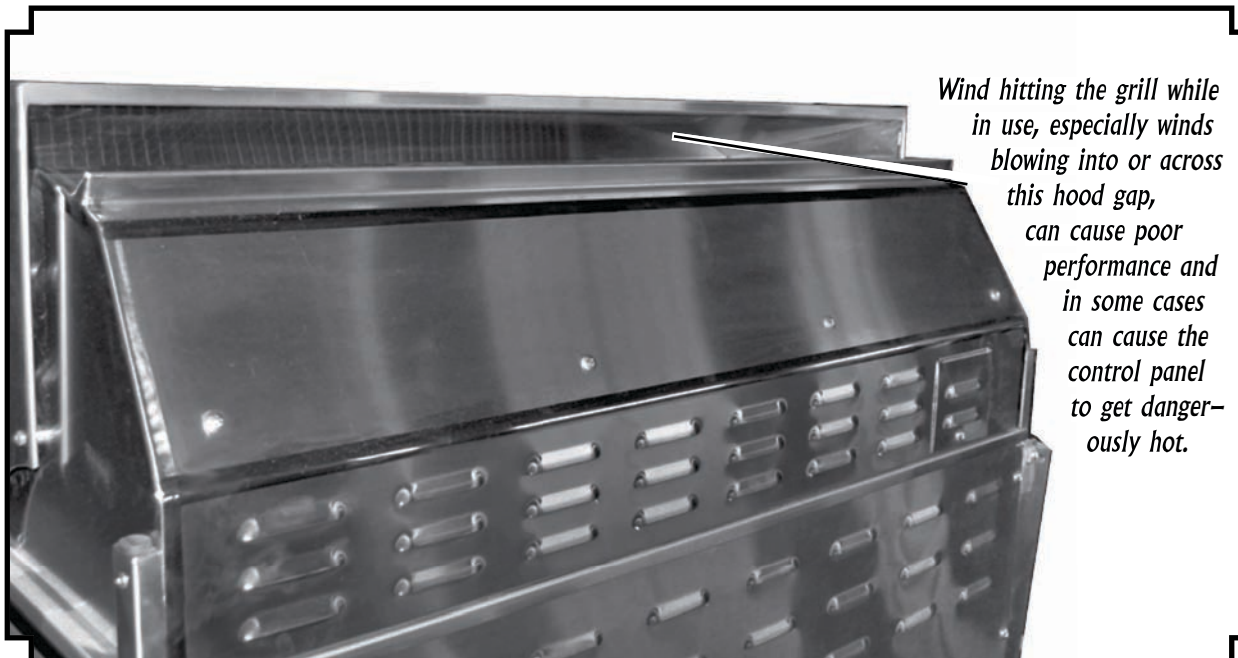
Figure 3-2 - Steady or gusty winds can prevent the normal exhaust of hot gases. Locate your grill away from prevailing winds and avoid grilling in windy conditions.
