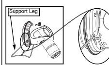
A wire Support Leg is supplied with your unit as an alternate means to support your heater.
