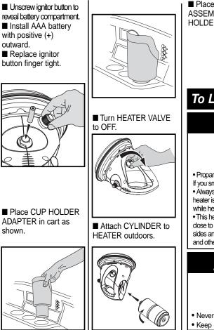
■ Place HEATER ASSEMBLY in CUP HOLDER ADAPTER.
