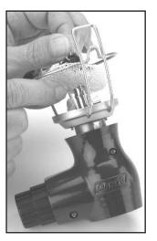
■ Make sure MANTLE is properly positioned with top and bottom in grooves of burner.
