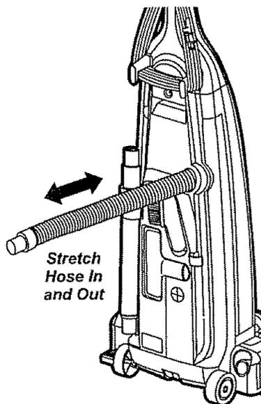
Plug in the vacuum and turn it on. Stretch the hose to maximum length and then allow the hose to return to its storage length.
