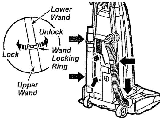
Unlock the wand by turning the wand locking ring to the **UNLOCK** position.
