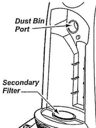
Remove any clogs that might be located in the dust bin port or the secondary filter.
