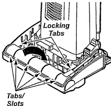
Lower the agitator cover to its original position. After positioning the agitator cover, push forward on the two (2) locking tabs in order to ensure that they are securely in place.
