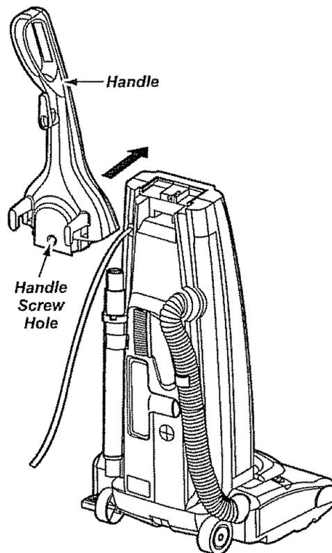
Insert the screw so it passes through the handle into the vacuum.
