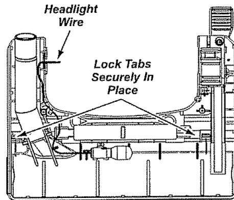
Make sure the headlight wires are tucked securely in place.
