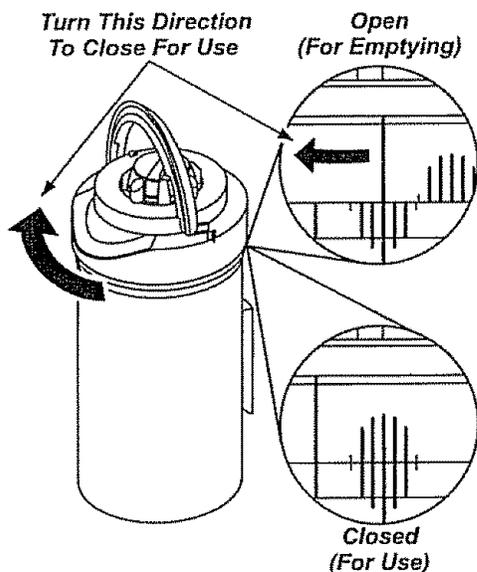
Replace dust bin lid assembly by placing back on dust bin with the marks on the lid aligned as shown under **Open (For Emptying)** on the back of the dust bin. Rotate lid clockwise while pressing downward so marks align as shown above **Close (For Use)** as above.
