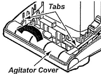
Depress tabs on rear of agitator cover and rotate forward to release from the nozzle body.
