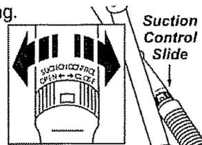
**NOTE:** Return suction control slide to the closed position for normal cleaning.
