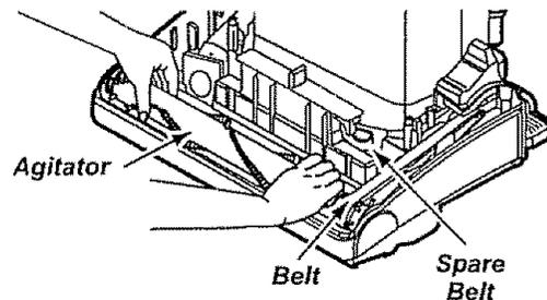
Position hands on the agitator. If the belt is still attached to the agitator, there will be tension on the agitator. Carefully lift the right end of the agitator and then the left end.
