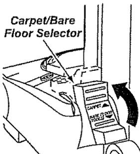
Place the carpet/bare floor selector in the carpet position and lower handle to lay vacuum flat.
