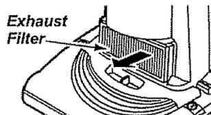
Remove the exhaust filter cartridge.
