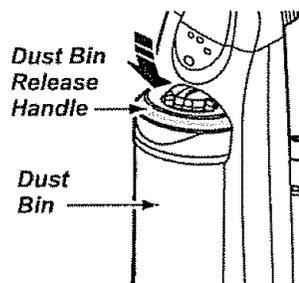
Lower the dust bin handle to lock dust bin in place.
