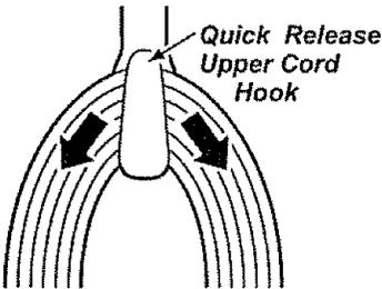
Turn the quick release upper cord hook to either side and down to release the power cord.
