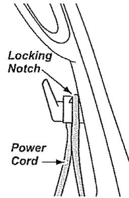
Wrap the power cord around the upper and lower cord hooks and lock the power cord plug onto the power cord.
