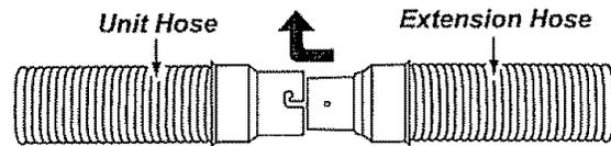
Insert the two tabs on the end of the extension hose into the two "J" shaped slots on the unit hose and twist to connect.
