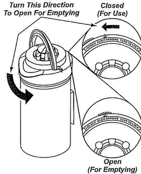
Rotate dust bin lid assembly counterclockwise as indicated on the lid and lift off.
