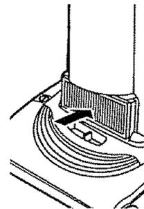
Replace the exhaust filter cover by placing tabs in slots and pushing in until cover snaps into place.
