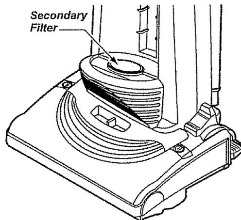
Wash the secondary filter in warm soapy water, rinse and dry thoroughly by squeezing the filter in your hand and letting it air dry.
