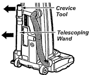
Remove the crevice tool from its storage position. Remove the telescoping wand from its storage position.
