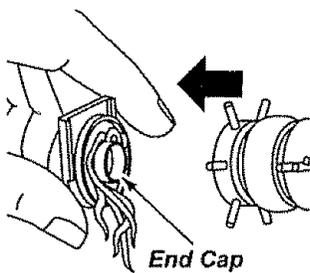
Carefully remove the brush end caps and remove any string or debris located on the agitator assembly, end caps or agitator shaft.
