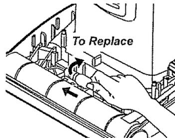
To replace the light bulb carefully insert and turn clockwise to securely fit into slot.
