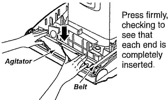
Press firmly, checking to see that each end is completely inserted.
