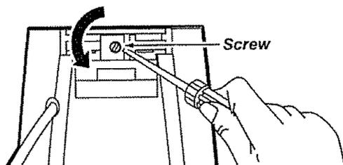
Remove the screw located just below the top edge of the back of the vacuum.
