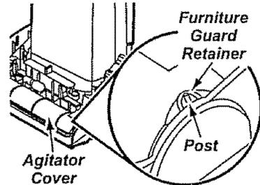
**NOTE:** If the agitator cover is not installed correctly, you may experience a loss of performance and possible agitator vibration, etc.
