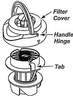
Replace dust bin lid by snapping into place with handle hinges aligned to tabs.
