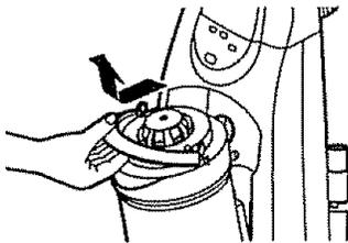
Pull the handle forward and lift dust bin up and out of the vacuum cleaner.
