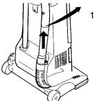
Remove the attachment hose from the lower hose retainer and look into the hose retainer for any obstructions. Proceed to Step 2 to check for any other blockages.
