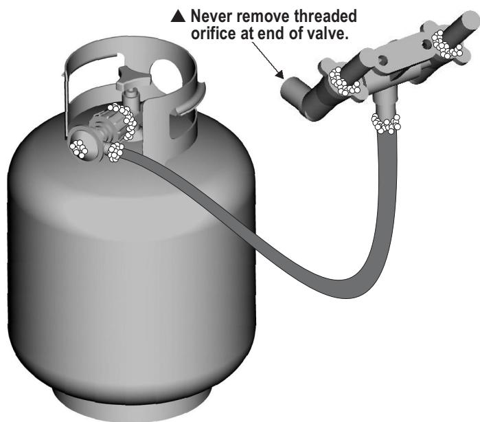
5. If “growing” bubbles appear, there is a leak. Close LP tank valve immediately and retighten connections. **If leaks cannot be stopped do not try to repair.** Call Sears for replacement parts at 1-800-4-MY-HOME®.
