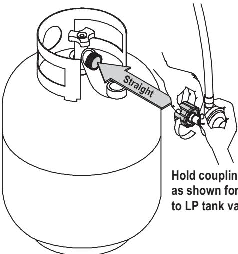
6. Turn the coupling nut clockwise and tighten to a full stop. The regulator will seal on the back-check feature in the LP tank valve, resulting in some resistance. **An additional one-half to three-quarters turn is required to complete the connection.** Tighten by hand only – do not use tools.
