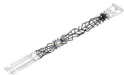
SPIDER AND WEBS INSIDE BURNER TUBE
