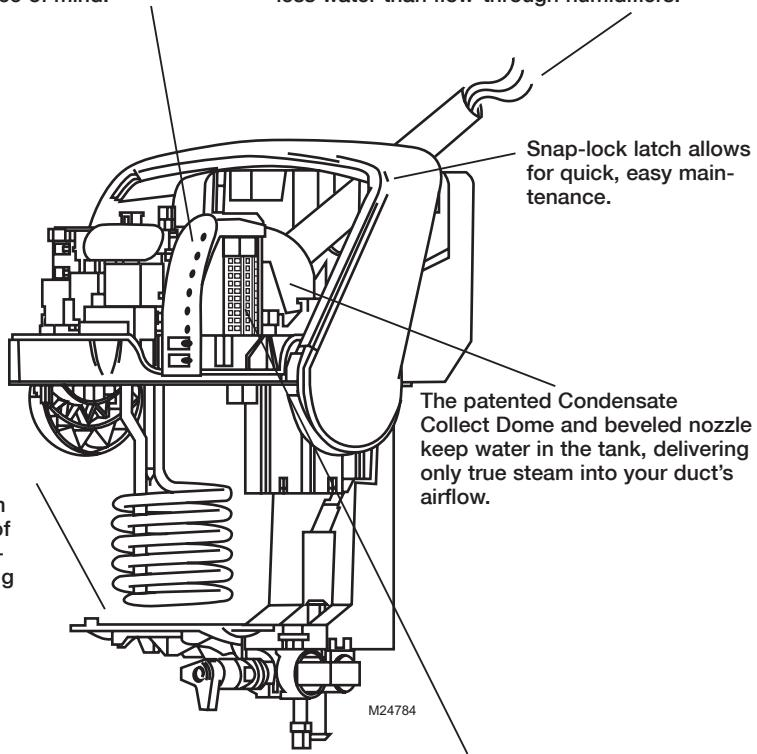
Automatically fills with water and drains when needed, so you don't have to remember to do it.
