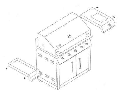
**Step 8:** Assemble push bar with ½"-20x1/2" screws to the left side shelf.
