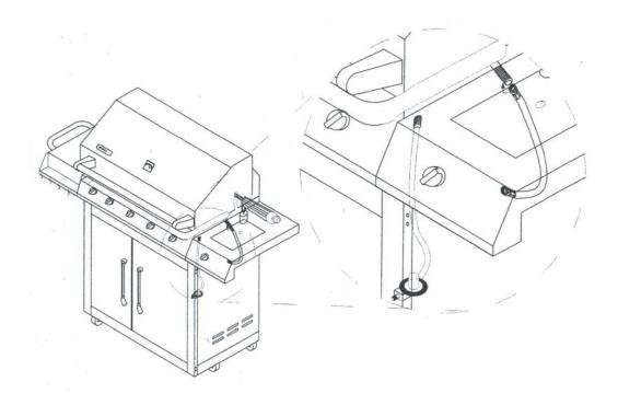
Step 10: Assemble the rotisserie kit as per the diagram below: First locate the motor bracket on left side of the bowl assembly with  $\frac{1}{4}$ "-20x1/2" screws. Then place the Motor onto the motor bracket and last assemble the rotisserie as the figure shows.
