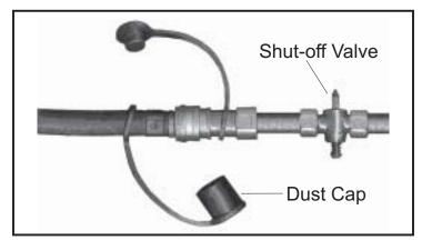
5. Push the plug into the connector until the sleeve snaps forward to lock the fitting in place. Turn on the shut-off valve. The flow of gas to the appliance will be restricted if the plug is not connected properly.
