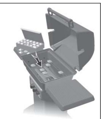
2. Open the package containing the ceramic briquettes and place them on the rock grate.
