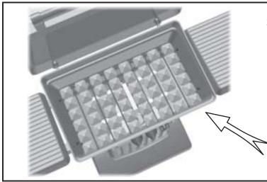
3. It is important to properly arrange all the ceramic briquettes onto the rock grate to allow for good air flow during use.
