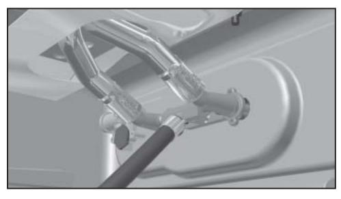
Improper installation and connection of the burner tubes to the control valves is dangerous and may lead to damaging fire and personal injury.
