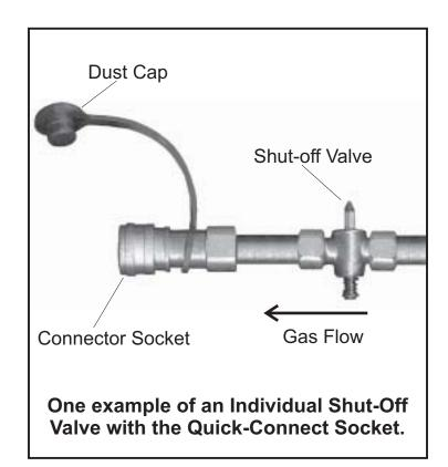
Prior to inserting, turn on gas supply and test all connections with an ammonia-free soap and water solution. Apply this solution to the stem of the shut-off valve and opening of the socket to detect leaks. (See Leak Testing Natural Gas Connections on the following page).
