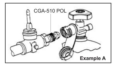
**Filling a Type 1 Cylinder Valve** Example A: shows a CGA-510 POL fitting. Example B: shows using a Type 1 POL fitting.
