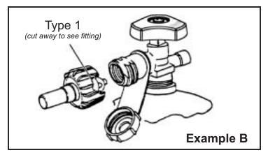
The L.P. gas cylinder has a Type 1 cylinder valve with a back-check module in its outlet that will not permit gas to flow until an evacuation device is installed. To purge the L.P. gas cylinder, the back-check module must be opened with an evacuation device.
