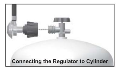
1. The top knob on the supply cylinder must be closed. See that the top cylinder knob is turned clockwise to a full stop.
