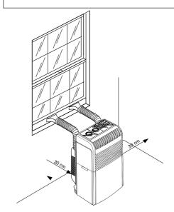
Vent holes for air discharge to the exterior can be made in any wall or window frame as shown in fig. A1, A2 and A3.
