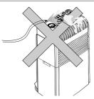
Under no circumstances should appliance be washed with running water. Damage could be caused to the electrical circuit.
