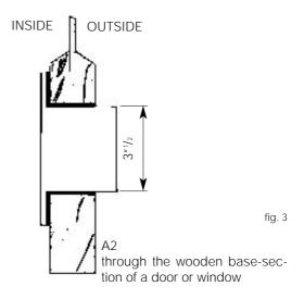
In case of fixed installation, air discharged from rear hose has been extracted from the room where the appliance is installed.
