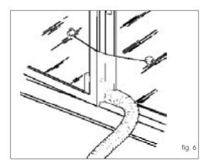
Pinguino is equipped with an adjustable window bracket. If you have a sash window, place the bracket on the window sill, extend the bracket fully within the window frame and lower the window onto the bracket. Insert the nozzle of the exhaust hose into the slot, then connect the hose to the air conditioner (fig.7). Thanks to the wing nut, it's possible to use the window bracket also for sliding windows. Position the hole of the bracket so to allow a correct installation of the exhaust hose.
