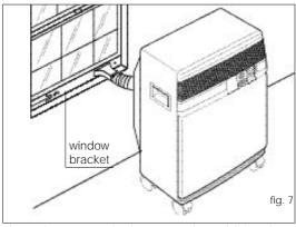
If you have a sash door, use the additional set provided in order to extend the accessory to the desired length; joining the two parts (fig. 8), adjust the total length according to your needs then, fix the bracket with the relevant nuts, close the door and connect the hose (fig. 9).
