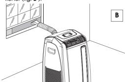
Thanks to the locking pins, it's possible to use the window bracket also for sliding windows. Position the hole of the bracket so to allow a correct installation of the exhaust hose (see figure **C**).
