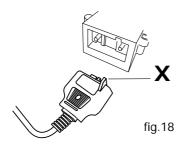
If the magnetic connector does not remain in place, check that it has been inserted correctly, see Figure 18. If the problem persists, contact an authorised service centre.
