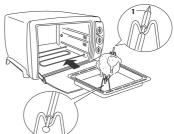
Place the dripping pan with the food being cooked in the lower guide (3), tilting the spit supports (Q) to the left. Make sure that the tip of the spit 1 is facing for-
