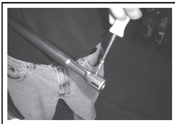
Loosen screw on air shutter. Tighten after adjusting.
