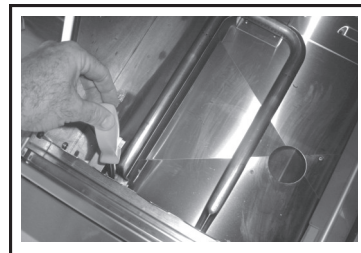
Install burner. Tighten screw.
