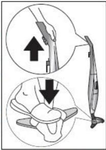
and pull the sweeper handgrip upwards until the brush joint is released.
