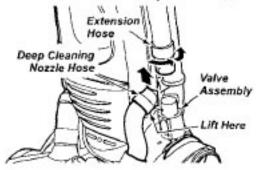
To clean the sensor, remove deep cleaning nozzle hose at valve assembly by lifting hose straight up. Remove extension hose from the valve assembly by grasping hose collar, twisting, and pulling straight off.
