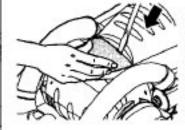
Replace light lens using a flat screwdriver to press the lens tabs into place.
