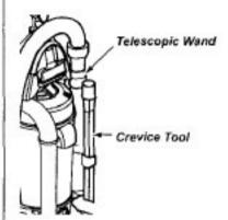
Remove the telescoping wand from its storage position by twisting and pulling out.
