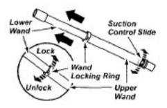
On the telescopic wand turn the locking ring clockwise to the UNLOCK position. Extend the wand to its full length, Turn the locking ring counter-clockwise to the LOCK position. Attach the extension wand onto the open end of the hose.
