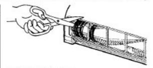
To clean agitator turn vacuum over, cut off any carpet pile and lint entangled around agitator with a pair of scissors in the slots provided. Remove hair, string, lint and other debris from the agitator.
