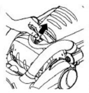
To replace the light bulb carefully insert securely into slot. Replace lens cover.
