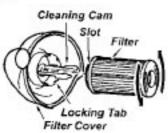
Clean primary filter by gently tapping over a trash container. Tap on several sides to ensure best cleaning. Rinse with water only as needed, do not use any detergent or soap. Allow the filter to dry for 24 hours before putting it back into the vacuum.
