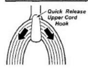
Turn the quick release upper cord hook to either side and down to release the power cord.
