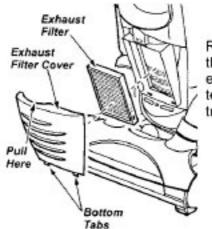
Remove the exhaust filter cartridge.
