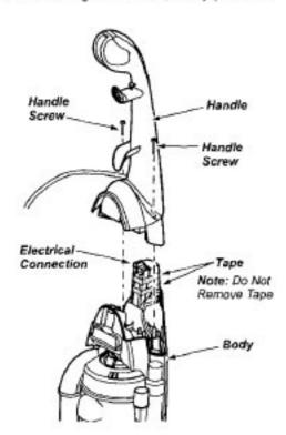
handle onto the body. Secure with handle screws provided.
