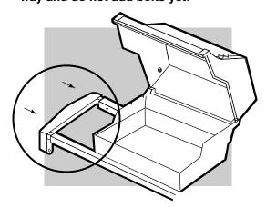
2.) Slide the swing-up work surface rod through the holes at the top of the swing-up work surface.
