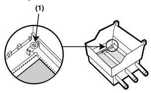
6) Lift and twist the burner assembly slightly, to separate the crossover tube(1) from the burners. Remove the burners from the cooking box.
