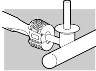
5) Remove the manifold bracket and unscrew the two wing nuts(1) that hold the manifold to the cooking box. Pull the manifold and valve assembly out of the burners and carefully set it down.
