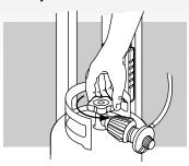
7) Check for leaks by wetting the fitting with the soap and water solution and watching for bubbles. If bubbles form, or if a bubble grows, there is a leak. If there is a leak, turn off the gas and tighten the fitting. Turn the gas back on and recheck with the soap and water solution.
