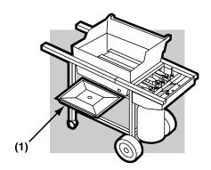
Put the disposable drip pan into the catch pan. Slide the catch pan into the catch pan holder with its finger grip towards you(1).
