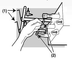
5) Slide the burner assembly out from under the guide screw and washer(1) in the corners of the cooking box.
