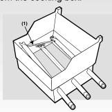
8) To reinstall the burners, reverse 3) through 7). \( \triangle \) CAUTION: The burner openings(1) must be positioned properly over the valve orifices(2). Check proper assembly before fastening manifold in place.
