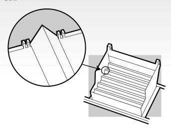
Set the cooking grates onto the ledges in the cooking box with the rounder sides up.
