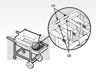
Slide the cylinder panel up until notch at bottom of panel fits over the cross brace(1). Add nylon washer to bolt and insert through the hole in the wheel frame at the bottom right of the cylinder panel, make sure that the bolt slips through the hole in the cylinder panel. Add nylon cylinder glide to bolt end and tighten bolt with the wrench, while holding the cylinder glide with the pliers. Repeat procedure with the hole on the bottom left side of the cylinder panel.
