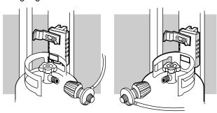
2) Loosen the cylinder lock wing nut. Swing the cylinder lock down. Tighten the wing nut.
