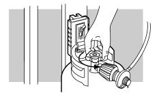
To perform leak checks: open tank valve by turning the tank valve handwheel counterclockwise. Check for leaks by wetting the connections with the soap and water solution and watching for bubbles. If bubbles form or if a bubble grows, there is a leak. Note - Since some leak test solutions, including soap
