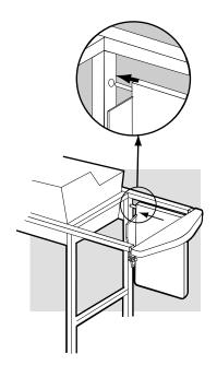
4.) While holding swing-up work surface in position, insert the other end of the swing-up work surface rod into the left end trim piece. Push the trim piece into the frame.
