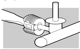
The Weber Spider Stopper™ Guard(1) is factory installed. It fits tightly around the air shutter section of the burner tube and the valve, thereby preventing spiders and other insects access to the burner tubes through the air shutter openings.
