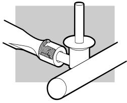
⚠ WARNING: After reinstalling the gas lines, they should be leak checked with a soap and water solution before using the barbecue. (See Step: "Check for gas leaks.")
