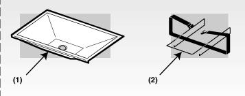
Hook the ends of the catch pan holder into the hole in the slide out bottom tray. The front of the catch pan holder must be on the same side as the finger grip(1) of the bottom tray.
