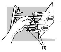
6) Slide the burner assembly out from under the guide screw and washer(1) in the corners of the cooking box.
