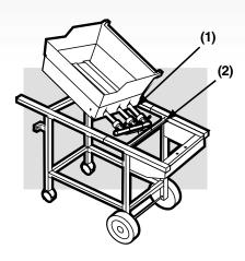
Slide the cooking box (assembly) to the left within the frame assembly. Add the nylon washer to the bolt. Insert the bolt through the frame and cooking box with the head of the bolt outside the box. Add the keps nut. Tighten by holding the bolt with pliers while you tighten the nut with a wrench.
