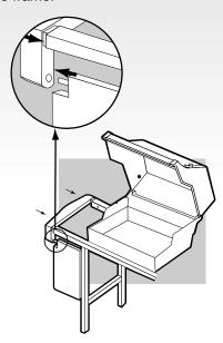
5.) Add a washer to each bolt and insert it through the hole in the frame and the hole in the trim piece on both sides. Tighten with a wrench.
