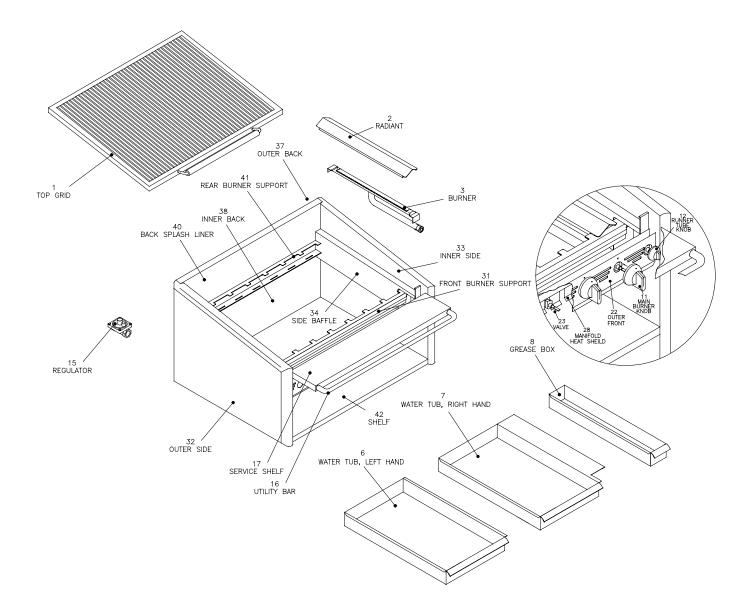
8. **TYPICAL SMB 600 SERIES ILLUSTRATION** (Model SMB 636 shown) Note: Your unit may vary from this typical diagram.
