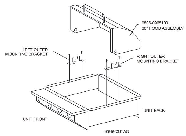
Mount a pair of outer hood brackets as shown. Lift the hood onto its brackets, making sure the pivot bushings sit in the bracket cradle on each side, as shown in the close-up illustration above.
