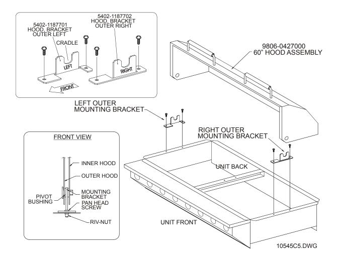
Mount a pair of outer hood brackets as shown. With a minimum of two persons, lift the hood onto its brackets, making sure the pivot bushings sit in the bracket cradle on each side, as shown in the close-up illustration above.
