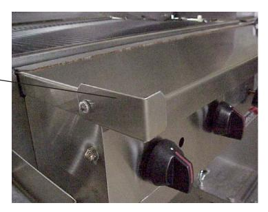
The cutting board lays inside the confines of the brackets in the front and the frame edge at the back.
