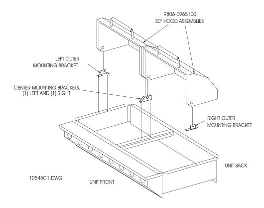
Mount a pair of outer and a pair of center hood brackets as shown above. Lift the hoods, one at a time, onto their brackets, making sure the pivot bushings sit in the bracket cradle on each side, as shown in the close-up illustration above.
