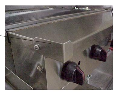
The cutting board lays inside the confines of the brackets in the front and the frame edge at the back.
