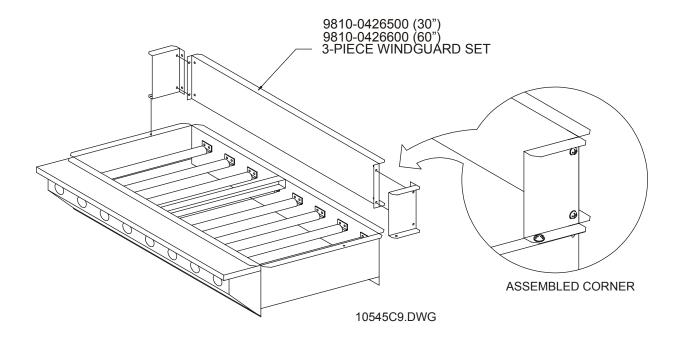
Assemble the Windguard ends to the back using the ½" long ¼-20 screws and the acorn nuts from the hardware bag in the Windguard package. Mount the Windguard on the charbroiler frame (either at the back or in the front) using the ¾" screws and the hex nuts, as illustrated in the close-up.
