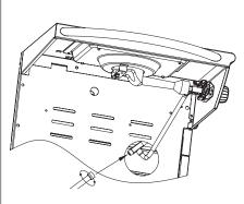
Attach the Natural Gas Hose (included with your barbecue) to the grill. Tighten the female nut of the hose onto the side burner valve using a wrench.
