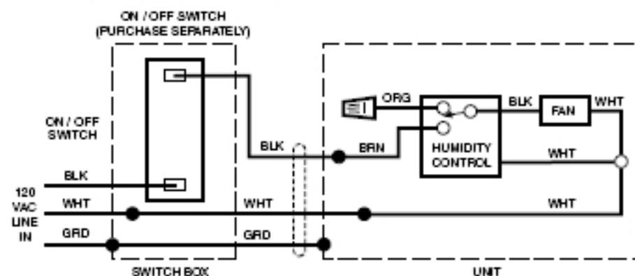
**WIRING OPTION #2** - Fan can be turned ON, OFF, or set to operate automatically.
