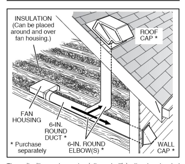
The unit will operate most quietly and efficiently when located where the shortest possible duct run and minimum number of elbows will be needed.
