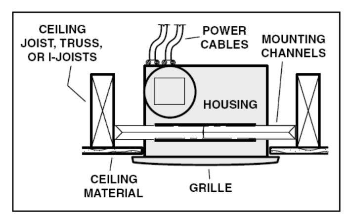
Housing mounted directly to joists, trusses, or I-joists. Up to 24-inches on-center.
