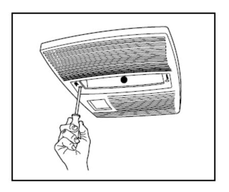
To avoid damage to the grille: DO NOT OVERTIGHTEN SCREWS. Tighten screws only until grille is snug against ceiling material.
