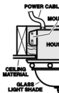
HOUSING MOUNTED TO ADDITIONAL JOIST Discharge parallel to joists.
