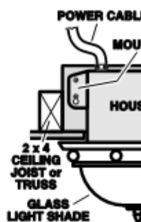
HOUSING MOUNTED TO 2x4 TRUSS Requires additional framing for mounting tabs. Discharge perpendicular to joists.
