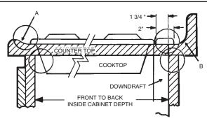
Refer to the cooktop installation instructions for dimensions of cooktop, countertop cut-out, and cabinet requirements. The RMDD3004EX can be installed in most standard 30" wide cabinets, (RMDD3604EX can be installed in most standard 36" wide cabinets), (RMDD4804EX can be installed in most standard 48" wide cabinets).
