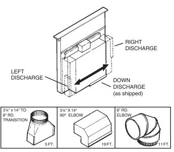
The system will operate most efficiently when the ductwork does not exceed 40 feet of equivalent duct. The chart above, shows equivalent feet of elbows and transitions. The number of feet of straight 31/4" x 14" or 8" duct plus the equivalent feet of elbows or transitions to be used should equal 40 feet or less.
