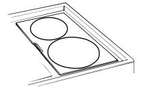
**3.** Lower the inside edge of the module into the cooktop until it is flush with the cooking surface.
