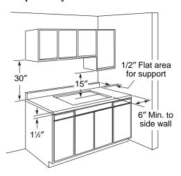
Avoid placing cabinets above the cooktop unit, if possible, in order to reduce the hazards caused by reaching over heated surface units. If cabinets are placed over the cooktop, the risks can be reduced by installing a range hood that projects horizontally a minimum of 5 inches beyond the bottom of the cabinets.
