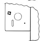
Feed the power supply leads through the conduit; be sure to leave enough length to properly connect these leads to the cooktop power leads.
