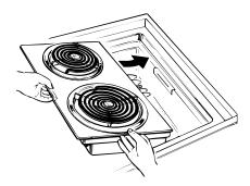
1. Be sure the controls are turned to OFF. To install the module, position the plug to the outside wall of the cooktop.
