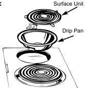
Repeated lifting of the surface unit more than 1 inch above the drip pan can permanently damage the receptacle.
