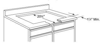
A 1/2" wide flat area is required around the edge of opening for support of the unit. The cooktop unit must be level and sit squarely into countertop opening.
