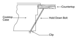
Secure cooktop by tightening hold-down bolts in bottom of the cooktop case. (2 bolts, 1 per side.)
