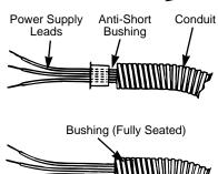
Thread the leads through an anti-short bushing and firmly seat the bushing in the end of the conduit.
