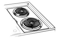
**3.** Lower the inside edge of the module into the cooktop until it is flush with the cooking surface.
