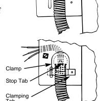
Tighten the clamping screw until the clamping tab is fully seated against the wire compartment.
