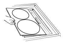
2. Slide the module toward the outlet in the side of the cooktop until the plug is pushed all the way in.
