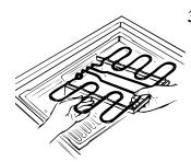
3. Make sure all controls are turned to OFF. Hold the heating element with the plug facing the side of the cooktop and level with the surface. Insert the plug into the cooktop outlet as far as it will go. (Do not force.) The heating element support should rest on the ledge of the reflector pan.
