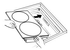
1. Be sure the controls are turned to OFF. To install the module, position the plug to the outside wall of the cooktop.
