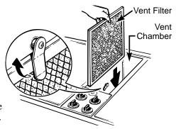
Clean the filter by swishing it in hot, soapy water. Rinse well and dry thoroughly.
