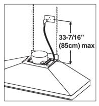
WARNING - Improper grounding can result in a risk of electric shock. Consult a qualified electrician if the grounding instructions are not completely understood, or if doubt exists as to whether the appliance is properly grounded. Do not use an extension cord. If the power supply cord is too short, have a qualified
