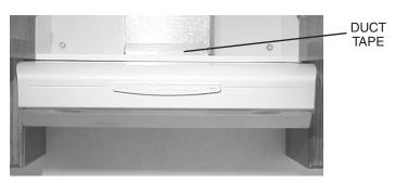
Connect ductwork to hood. Use **<u>Duct Tape</u>** to make joints secure and air tight.
