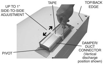
3¼" x 10" Ducted Discharge Only: Remove <u>Tape</u> from damper flap and attach <u>Damper/Duct Connector</u> over knockout opening with screws removed in Step 4 under "PREPARE THE HOOD". Make sure damper <u>Pivot</u> is nearest to <u>Top/Back Edge</u> of hood.
