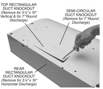
Remove appropriate **<u>Duct Knockout(s)</u>** from top or back of hood.
