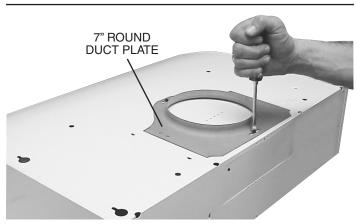
Remove <u>7" Round Duct Plate</u> from top of hood. Set duct plate aside - with mounting screws.
