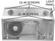
Remove <u>Light Panel</u> - held in place with (3) #8 screws and (2) #8 screws. Disconnect light assembly wire harness (white connector).
