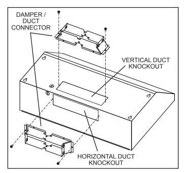
Remove <u>Vertical Duct Knockout</u> or <u>Horizontal Duct</u> <u>Knockout</u> and attach <u>Damper / Duct Connector</u> with two (2) screws (supplied).
