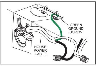
9 Connect <u>House Power Cable</u> to range hood wiring - BLACK to BLACK, WHITE to WHITE, and GREEN or BARE WIRE to <u>GREEN Ground Screw</u>.
