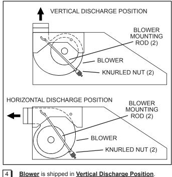
Blower is shipped in Vertical Discharge Position.
