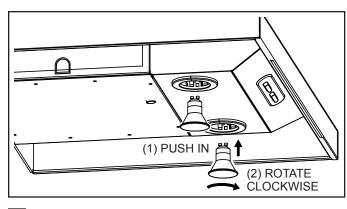
Install <u>Halogen Bulbs</u>. Use 120 V, 50 W, shielded halogen bulbs - MR16 or PAR16 with GU10 base. Purchase bulbs separately.
