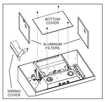
3 Remove the Aluminum Filters, Bottom Cover, and Wiring Cover from the hood.
