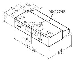
Rectangular Vented — 3-1/4" x 10" vertical or horizontal. Remove knockout #2 for vertical or knockout #3 for horizontal venting. Install damper/duct connector over opening. Go to "Planning Ductwork Installation".
