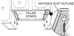
6. Screw the four supplied screws for mounting the hood into the exact center of the narrow end of the keyhole slots marked underneath the cabinet. Allow 3/8" of the screws to project, so the hood can be fitted into place.
