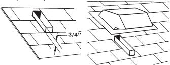
Roof Cap Discharge: Cut a hole in roof slightly larger than duct size being used. Trim shingles around hole so that they will fit snugly around hood of cap when cap is installed. Assemble the ductwork and tape all joints. Run ductwork down to hood location. Make sure that enough duct runs into the room so that the duct will overlap damper/duct connector when hood is put into place. Leave 3/4" of duct projecting above roof surface on high side.
