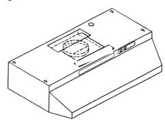
Round Vented — 7" vertical. Remove knockouts #1 and #2 exposing duct collar. Go to "Planning Ductwork Installation".
