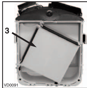
3) Heat recovery core
