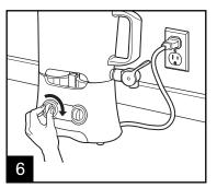
When using 80-ounce jar, only use **ONE** control knob to run **BOTH** blades: **1** (Low), **2** (High), or **P** (Pulse).
