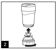
Cutting assemblies should be removed from 80-ounce jar and used with Personal Blending Jar.
