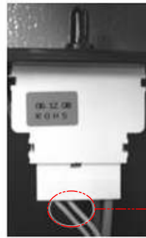
CON9 (PIN4&3) CONNECTOR 9 R-DOOR S/W BO, PK PIN 3&4
