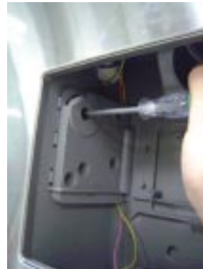
20) Sensor box can be disassembled after removal of 3 screws in same case of motor box.
