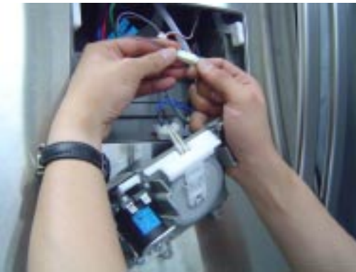
15) All harness have to be separated.
