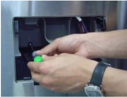
7) Unscrew 2 points to separate tray-cover
