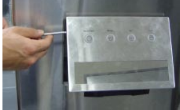
2) Unscrew left and right side (cross driver)
