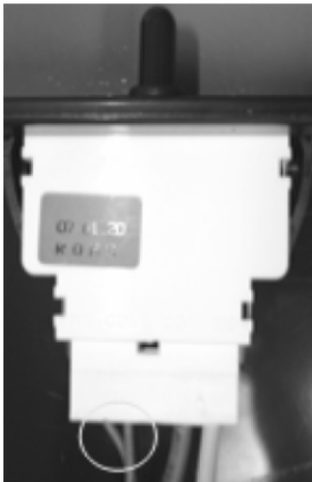
CONNECTOR 7 F- DOOR S/W 2*RD PIN 5&6
