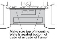
14. Slide washer onto holding pin and set inside upper cabinet.
