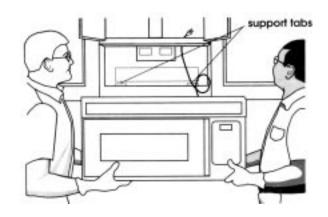
15. Carefully lift microwave oven hood and hang it on support tabs at the bottom of the mounting plate. Thread power supply cord through the power supply cord hole in the bottom of the upper cabinet.
