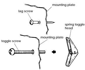
12. Insert lag Screws (into wall stud) or toggle bolts (through drywall) through the holes on the mounting plate at holes "A", "B", "C", "D" and "E".
