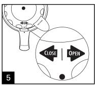
Align with open lock and twist to lock in place.
