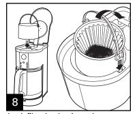
Lock filter basket into place. **IMPORTANT**: Lid will not close all the way if filter basket handle is not locked securely into place. 5
