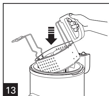
13 Holding Main Basket Handle, tilt Food Basket UNDER metal tab of Tilt & Hold Basket Hook.
