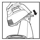
the back of the mixer onto the platform until it locks in position. The mixer can now be used as a stand mixer.
