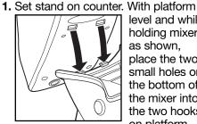
level and while holding mixer as shown, place the two small holes on the bottom of the mixer into the two hooks on platform.
