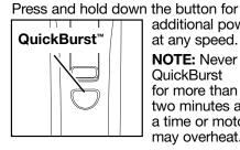
additional power at any speed. NOTE: Never use QuickBurst for more than two minutes at a time or motor may overheat.
