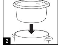
Carefully place cooking pot straight down on base. Make sure cooking pot is securely seated by rotating the pot left and right. NOTE: Make sure bottom of cooking pot is not bent or warped, or it will not conduct heat correctly.
