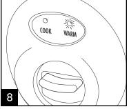
When finished cooking, cooker will automatically switch to WARM and light will glow.
