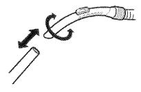
To remove handle: Pull up on handle by twisting slightly.
