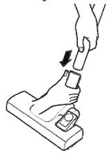
Push floor selector switch back for bare floor and forward for carpet. Brushes should be down for bare floor and up for carpet.
