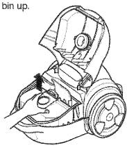
4. Hold the handle of the washable filter and pull it out of the dust bin.
