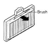
7. Pull the mesh screen down from the washable filter.
