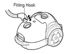
Insert hose into canister until it snaps into place.
