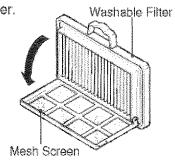
Clean the washable filter and the mesh screen with the brush under cold running water.
