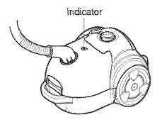
NOTE: Indicator may turn red when using attachments or when cleaning new carpet. This is due to reduced airflow caused by the vacuum seal between attachment and surface, or new carpet fuzz filling the dust bin quickly. Restore airflow by raising attachment slightly from surface you are cleaning, or empty dust bin if it is full.
