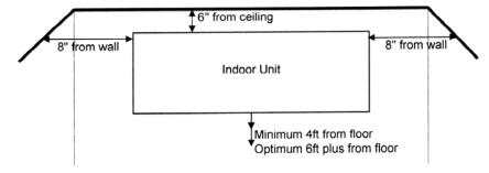
Ensure no obstacles to Airflow are directly in front of the unit, for a minimum of 12ft. for 9/12,000 Btu/h units and 16ft. for 18/24,000 Btu/h units. Do not install the Indoor unit units in areas exposed to high humidity (RH of 80% plus), direct sunlight and direct heat from stoves or other devices.
