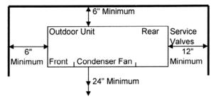
Install the Outdoor unit on a Condenser Pad or if a Heat Pump use feet to raise unit up approx 6" to allow for defrost to drain away
