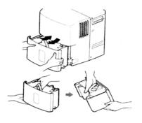
The bucket has a threaded hose connection which can be attached permanently. Remove cap on side of tank and attach a section of hose to the threaded connection and direct to desired area, or drain.
