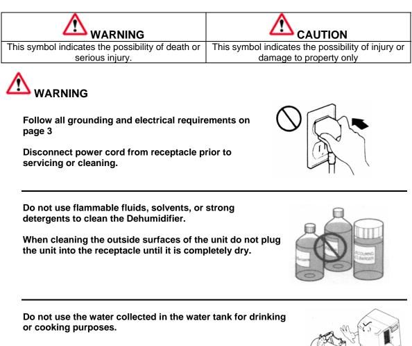
Do not clean the dehumidifier while it is plugged in. This can cause electrical shock.
