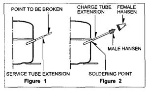
It is necessary to execute the soldering operation with valve open so that the fumes caused by oil residue can come out freely without blowholes between two tubes during the heating the of the point to be soldered. The extension fitted with the male Hansen is connected to the female fitting of the vacuum pump tube. (Figure 3)
