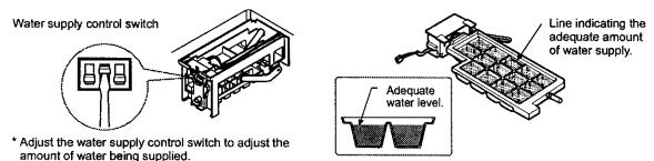
\* Make sure it is adjusted to meet the line indicating the adequate amount of water supply.
