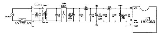
The secondary party of transformer consists of power (12Vdc) for driving display and relay and power (5Vdc) supplying power to MICOM and IC.
