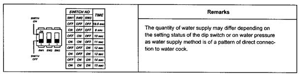
3. The change of the quantity of water supply setting may be done according to the changed time even after changing it without powering off. In the change of dip switch during water supply, it is done according to the water supply time previously established and then done according to the additionally changed time from the next water supply.
