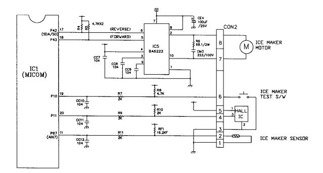
This circuit is a circuit used to embody functions such as ice-removing, full-ice detection, level noise, and ice-making temperature detection of ice-making tray (ice-making container).
