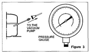
Air evacuating from the system begins as soon as the pump starts. The refrigeration system must be kept under vacuum until the reading on the low-pressure gauge indicates vacuum (0 absolute, -1 atm., -760 mm hg). In any case it is advisable to keep the pump running for about 30 minutes. (Figure 3)
