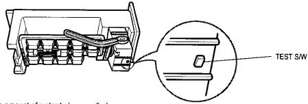
\* To check on the amount of water being supplied, press the Test button. (Hold for 0.5 seconds)
